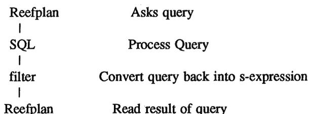
A simple timing test on a relation of 18,000 records each with 3 fields produced a retrieval rate of 41 records/second. By comparison the SQL interface to Mu-Prolog [1] retrieved 17 tuples/second on the same data.
